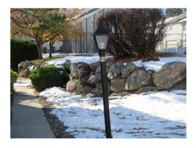
**Description:** Estimated 110 pathway pole lights. The lights have a 6-foot tall metal pole with lantern type light housing attached to the top of the pole. The majority of the pole lights are anchored in concrete with several anchored with soil.
